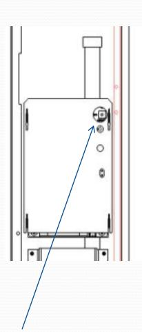
PRESS SERVICE MODE BUTTON AND ENTER TUBE FILL MODE (PRESS 1)
